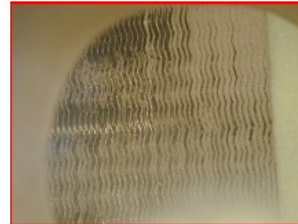
CO 2 freezes on cooling fins
