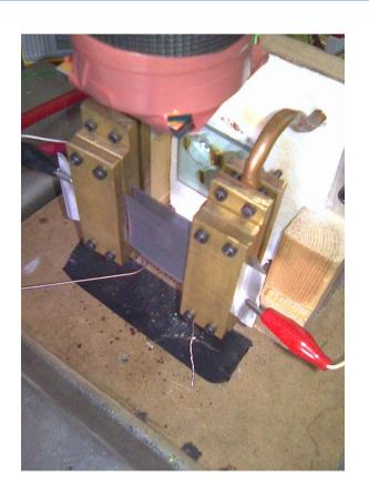
Vertically orientated wire mesh designed to heat a thermocouple (positioned near particle) to 900°C.
