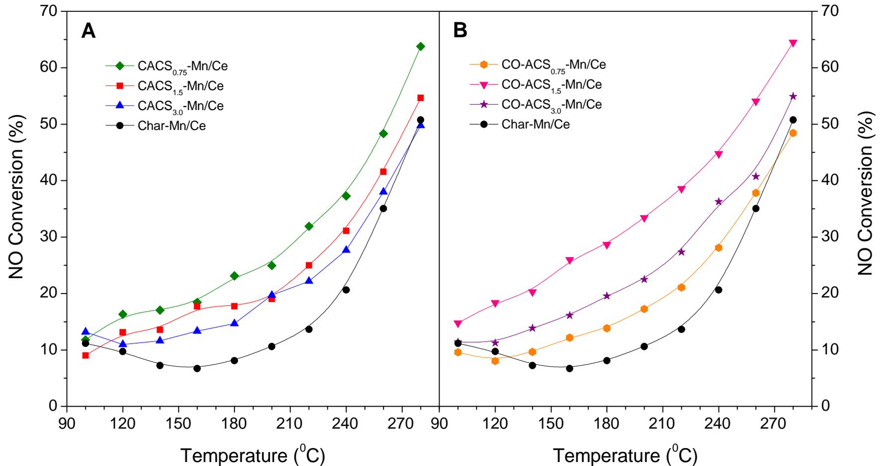
NO conversion (%) of chemically activated (CACS<sub>x</sub>-Mn/Ce) and co-activated (CO-ACS<sub>x</sub>-Mn/Ce) cotton stalk derived SCR-deNO<sub>x</sub> catalysts impregnated with Mn/Ce. A = CACS<sub>x</sub>-Mn/Ce, B= CO-ACS<sub>x</sub>-Mn/Ce.
