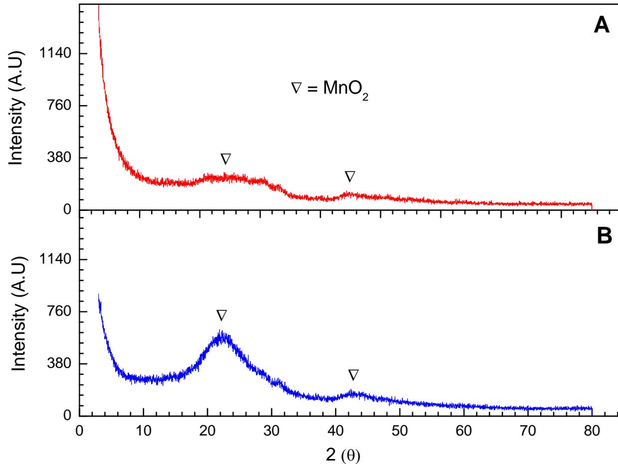
X-ray diffraction patterns of chemically activated ( $\text{CACS}_x\text{-Mn/Ce}$ ) and co-activated ( $\text{CO-ACS}_x\text{-Mn/Ce}$ ) cotton stalk derived SCR-de $\text{NO}_x$  catalysts impregnated with Mn/Ce. A =  $\text{CACS}_{1.5}\text{-Mn/Ce}$ , B =  $\text{CO-ACS}_{1.5}\text{-Mn/Ce}$ .
